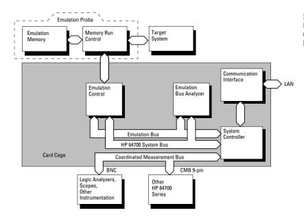
HP 64700 Series development tools include an emulator, an emulation bus analyzer, and an optional software performance analyzer (SPA).
